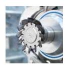
The underwater pelletiser is energy-saving, features a simple start-up procedure and can replace the strand pelletiser or automatic strand pelletiser. Pellet size and bulk density are adjustable for all pelletising systems.
