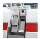
The high-vacuum degassing extruder reduces viscosity loss during extrusion and purifies the melt from volatile contamination. The waterfree vacuum pump reduces production and maintenance costs.
