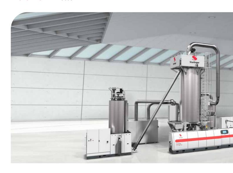
**State-of-the-art recycling** technology for the in-house recycling of PET flakes from bottles, preforms, strapping bands and sheets as well as for the recycling of post-consumer bottle flakes after the washing process. The end product is melt-filtrated, uniform granulate that can be used for a wide range of applications.
