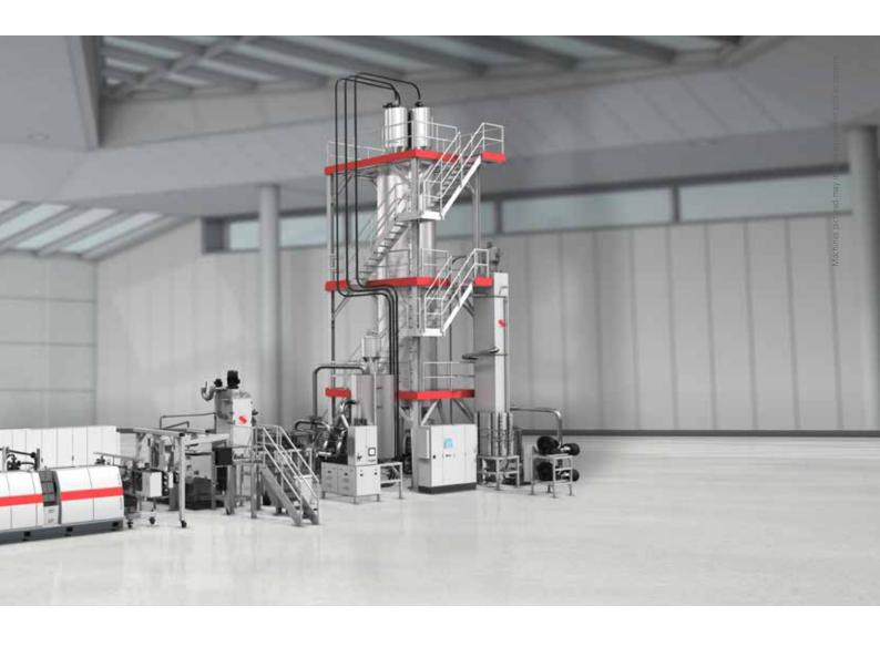
**Solid state polycondensation** – optionally for the **IV increase of PET and outstanding decontamination.** The regranulate after the Starlinger iV+ process is suitable for **food contact applications** such as bottle-to-bottle or bottle-to-sheet. The process has achieved several national and brand-owner approvals.
