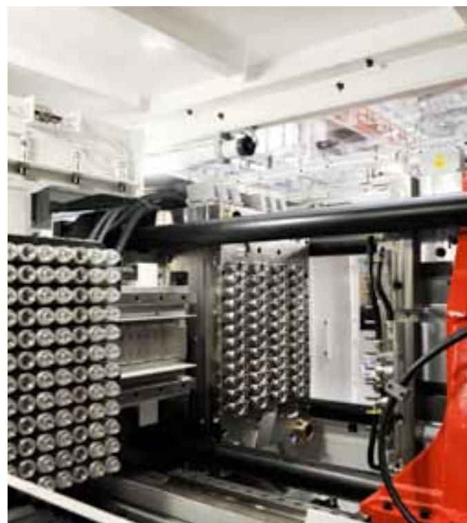
**EN** The new take-out robot is fully integrated into the injection machine. The preform post-cooling is made entirely in the robot hand. This solution ensures a better final preform quality, avoiding any risk related to warm handling.
