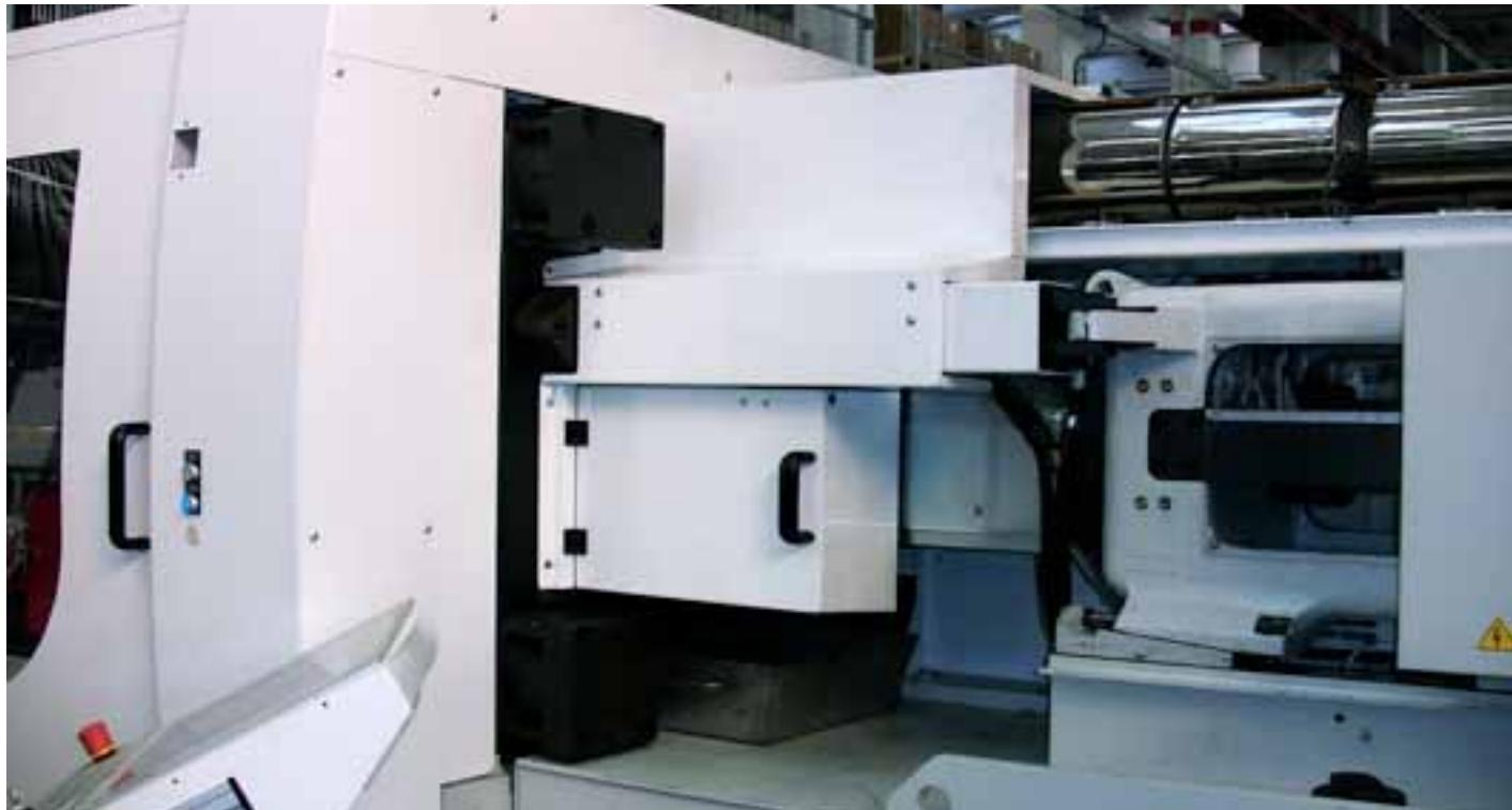
**EN** The injection system is composed by a plasticising cylinder with electrical drive screw, and an injection cylinder (shooting pot) driven by servo valve. This solution ensures high performances and machine energy saving.
