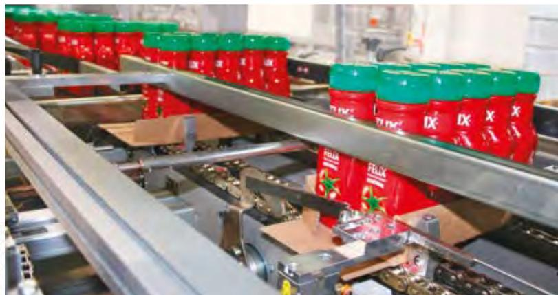
capacity of the container that is being used). Apart from the above mentioned, we have also recently added the CWP ERGON wrap-around case packers, these can produce up to 40 packs/minute and the new CM FP ERGON combined packer which was designed for packaging in film-only, pad + film, tray + film, tray-only and wrap-around case: all this from a single machine.
