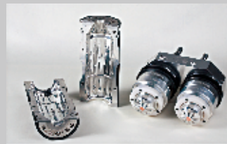
Blow mold of 500ml aseptic bottle for SIG/KHS machine
