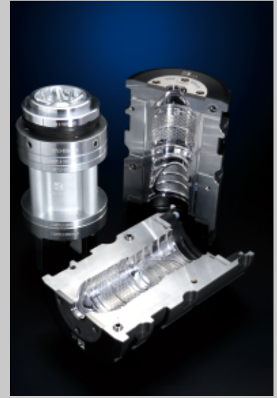
Blow mold of 550ml water bottle for SIDEL machine
