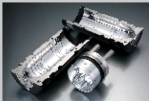
Blow mold of 2000ml CSD bottle for SIDEL machine
