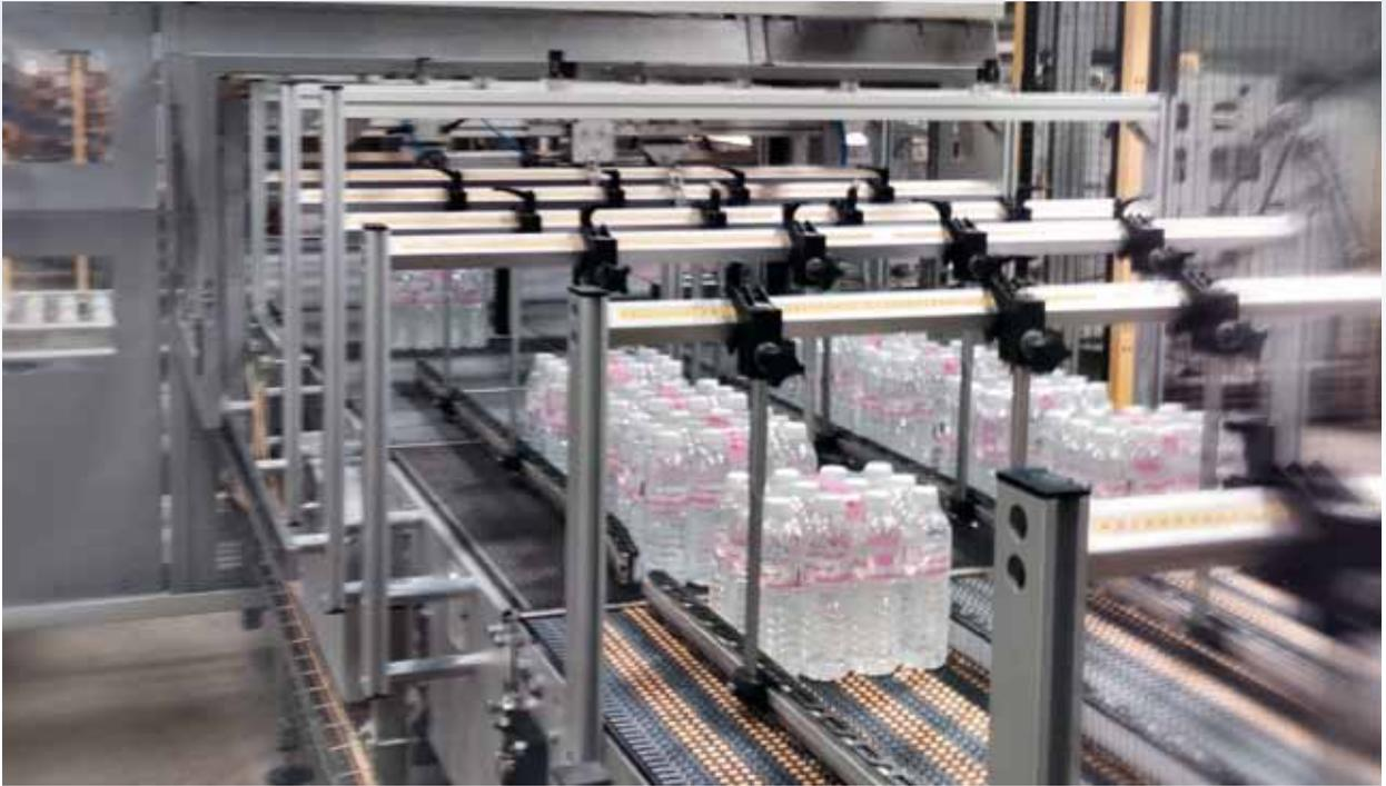
The central column of the APS 3070 P palletizing system is run by brushless motors, which guarantee highly dynamic, reliable and accurate movements of the operating axes.
