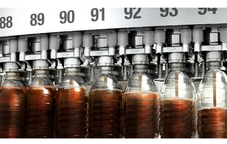
Aseptic filling technology aims at reaching the best performance in terms of filling speed, accuracy, flexibility and, at the same time, maintaining the sterility of the product: GEA Procomac aseptic fillers are designed focusing on the elimination of any possible risk for the product and crucial attention to environmental control.
