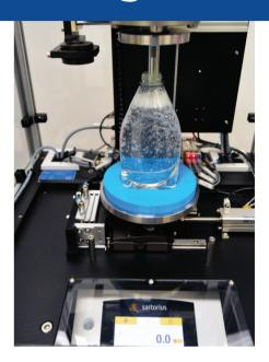
Torus Measurement Systems brings the world's first single operation Top Load & Volume Test, preventing the need for the operator to move the bottle between tests, and advancing the speed and accuracy of your quality checks. Suitable for use in production or Research & Development.
