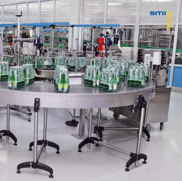
and glass (0.355-liter, 0.75-liter and 1.0-liter bottles) in wrap-around cardboard boxes with and without the preformed cardboard separators.
