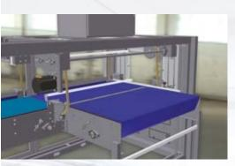
The APS 1550 P PLUS palletizing system satisfies production requirements up to 50 packs per minute (about 150 layers per hour) and can handle 800x1200 mm (europallets) and 1000x1200 mm pallets.
